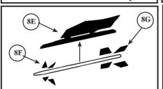
Sidewinder Missiles can be made for the Sea Harriers, using 10 thou wire or plastic rod in conjunction with the fins supplied as etched parts 8F and 8G.
