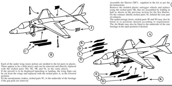
Wing Flaps Outrigger Wheels Aerodynamic Strakes Sidewinder Missile Pylon
