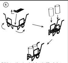
Fold the two side sections of etched part 6 to  $90^{\circ}$  on the front cross bar, so that they are parallel. Fold up the front retaining rail to  $90^{\circ}$  on the floor panel and fit between the two sides as shown. Cut two 2mm lengths of 1mm plastic rod or sprue to make the fluid containers. Fit these onto the trolley floor as shown above.
