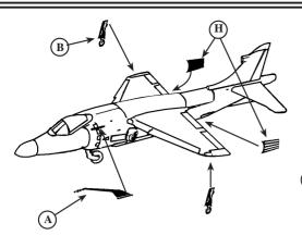
Each of the under wing stores pylons are molded to the kit parts in plastic. These appear to be a little heavy and can be removed and directly replaced with the etched parts 8D and 8E, in the same place. If the aircraft is to be displayed launching or landing, the wing flaps can be cut from the wings and replaced with the etched parts 8C, in the lowered position.
